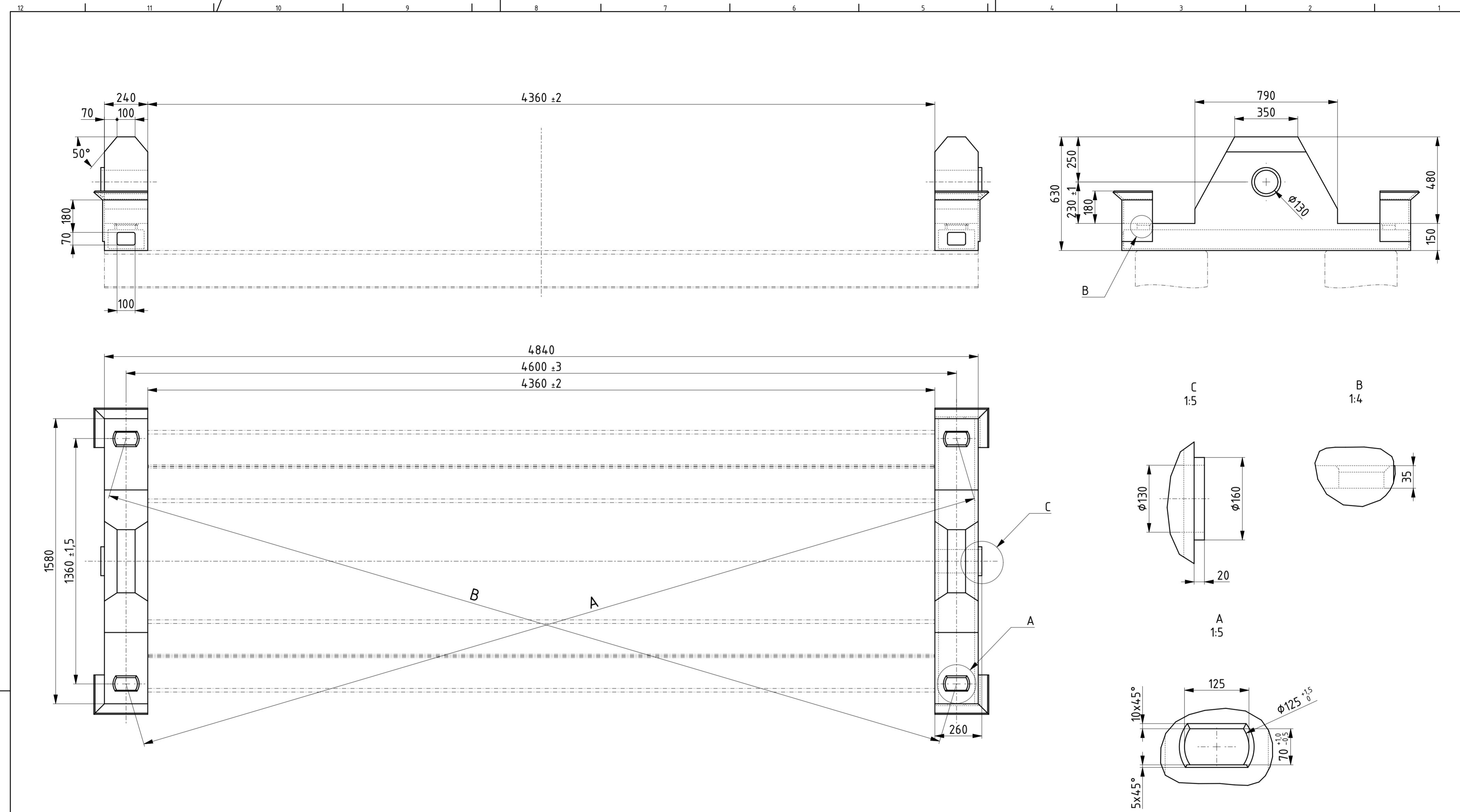
Difference between cross dimensions (A-B) max 4mm
