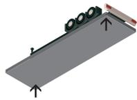
Before loading/unloading prepare the vehicle: close the cabin side-skirts, open twist-locks and watch out for any disturbing objects.
