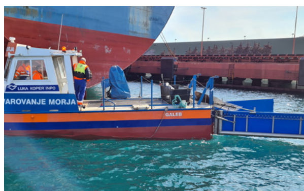
Demonstration of the cleaning of debris at the outlet of the river Rižana into Basin II of the port of Koper, placement of absorbent booms and cleaning of the sea surface with the eco-vessel Galeb.
